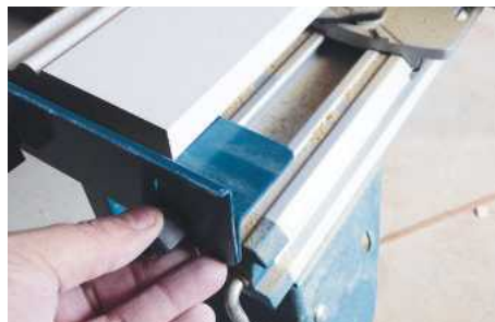
▲ A simple stop on the extension arm can be engaged by sliding it upwards
